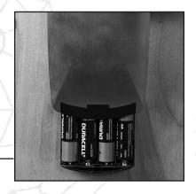
Secure the Battery Pack in the Inside Cover using one (1) flathead M4x12 hex screw. After the screw is fully tightened, loosen the screw by one full turn.
