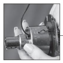
Insert the Adjustment Tool into the small hole of the Lock Motor and rotate the plate to the appropriate door thickness mark.
