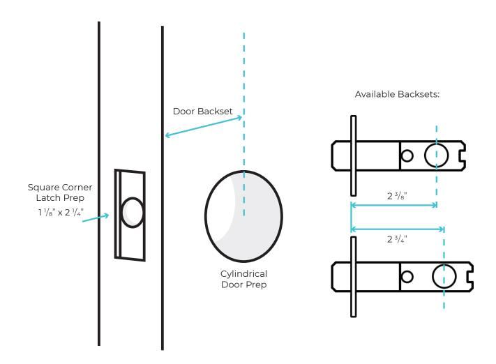
Door backset is the measurement from the door edge to the center of the cylindrical door prep or existing door knob.
