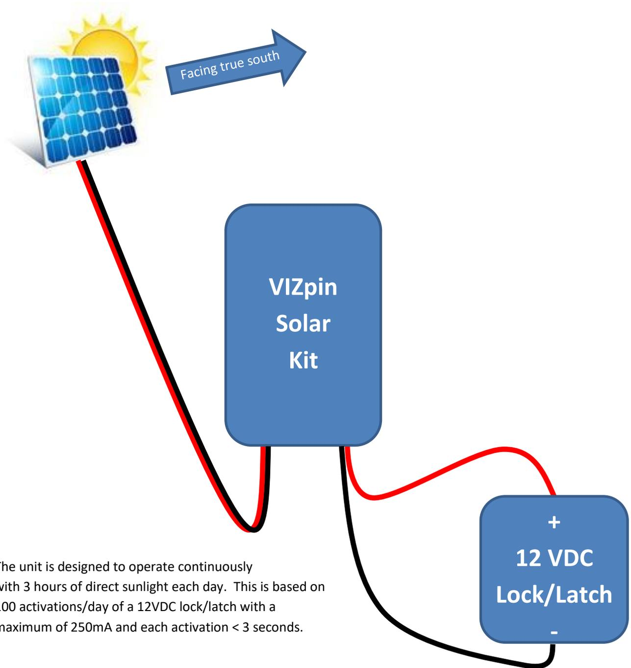
The unit is designed to operate continuously with 3 hours of direct sunlight each day. This is based on 100 activations/day of a 12VDC lock/latch with a maximum of 250mA and each activation < 3 seconds.
